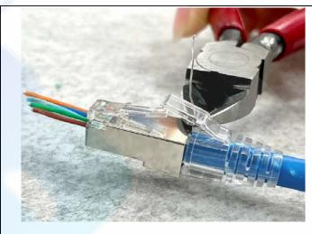
9. Cut the exposed drain wire. Slide the boot (optional) on and seat it firmly.
