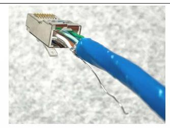
7. Set the drain wire at appropriate position to contact with external ground shield.
