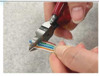
6. Untwist each pair downward towards the cable jacket and arrange in the T568B sequence. Flush cut the conductors in the front to have a uniform appearance.
