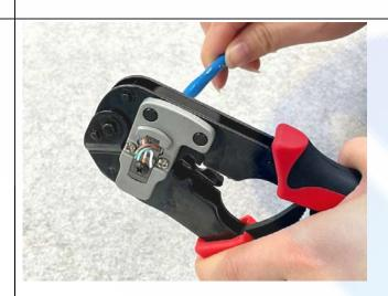
10. Terminated contact chips, cable holder and cut off exposed conductor by the crimp tool.
