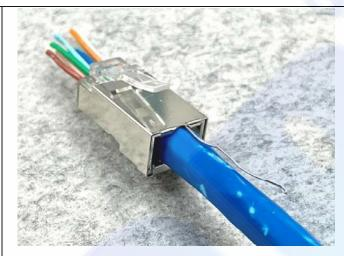
8. Insert the prepped wires into the connector let the wire thru the plug. For strength of connection, also push as much of the cable jacket as possible into the connector.
