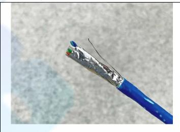
3. Expose the shield layer and drain wire.
