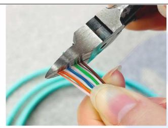
4. Untwist each pair downward towards the cable jacket and remove kinks from the conductors. Arrange in the T568B sequence. Flush cut the conductors in the front to have a uniform appearance.
