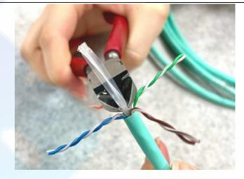
3. Place the conductor pairs into a "star" pattern at a near 90-degree angle to the cable jacket. Cut the cross divider.
