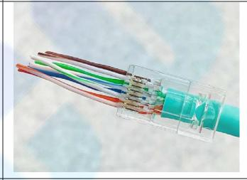
5. Insert the prepped wires into the connector and let the wire thru the plug. For strength of connection, also push as much of the cable jacket as possible into the connector.
