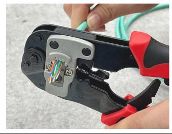
7. Terminated contact chips, cable holder and cut exposed conductor by the crimp tool.
